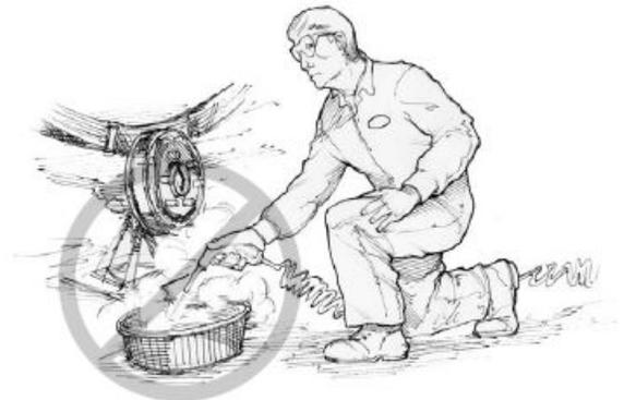
Never use compressed air to remove dust from automotive friction materials. Even if the employee shown here was wearing a respirator, others would still be exposed to airborne asbestos dust.
