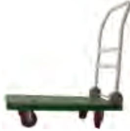
Flatbed Hand Truck Used to reduce carrying distance and frequency.
