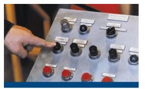
8. Push the stop button again, after you have tested for power. You don't want the machine to be in the "on" position when the power is turned back on at the main power disconnect.
