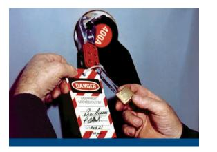
6. Release all stored energy from the system. Depending on the type of machine, there **may** still be several kinds of energy remaining after the power is turned off. The written lockout procedure should have a complete list of all these secondary energy sources and how to release energy from them.
