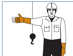
▲ Raise boom and lower load Relever la flèche et descendre la charge
